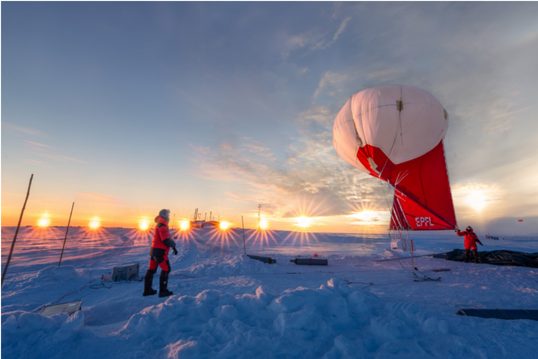
In spring 2024, Julia Schmale's team used a tethered balloon to measure aerosol-cloud interactions at the Villum research station in northern Greenland (82°N).
